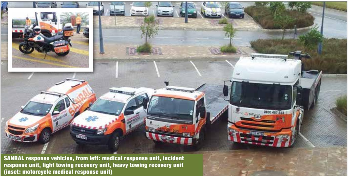
**SANRAL response vehicles, from left: medical response unit, incident response unit, light towing recovery unit, heavy towing recovery unit (inset: motorcycle medical response unit)**
