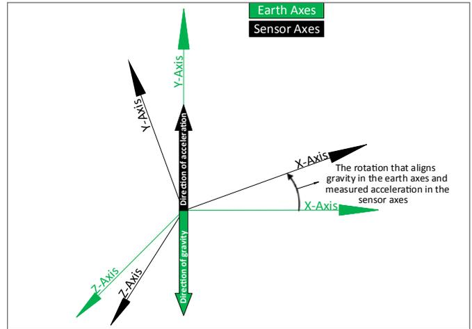
Figure 3: An illustration of the rotation  $q_E^S$  and how it is estimated using an accelerometer reading
