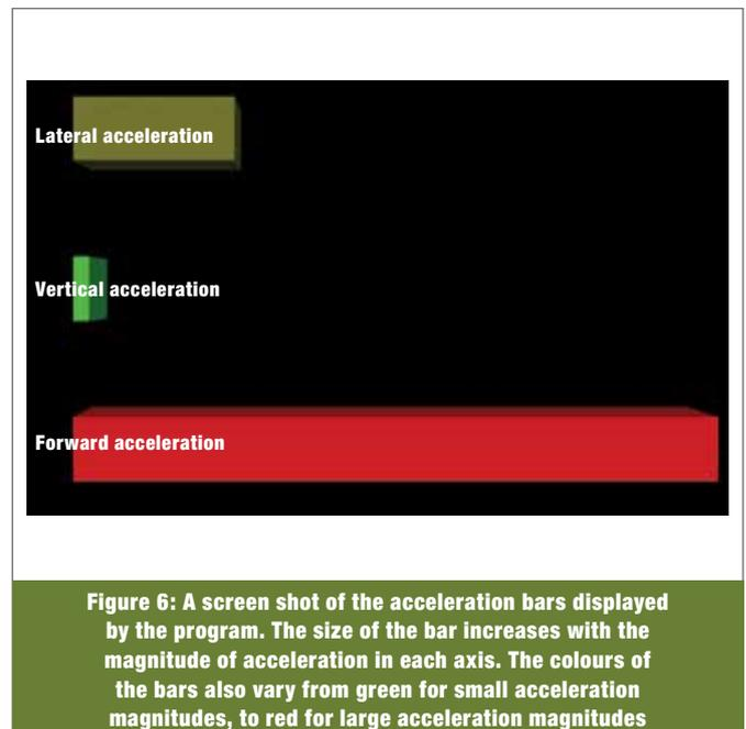
Figure 6: A screen shot of the acceleration bars displayed by the program. The size of the bar increases with the magnitude of acceleration in each axis. The colours of the bars also vary from green for small acceleration magnitudes, to red for large acceleration magnitudes
