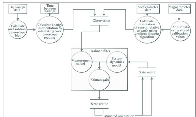
Figure 4: A data flow diagram illustrating the underlying flow of data within the system
