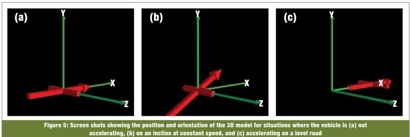
Figure 5: Screen shots showing the position and orientation of the 3D model for situations where the vehicle is (a) not accelerating, (b) on an incline at constant speed, and (c) accelerating on a level road
