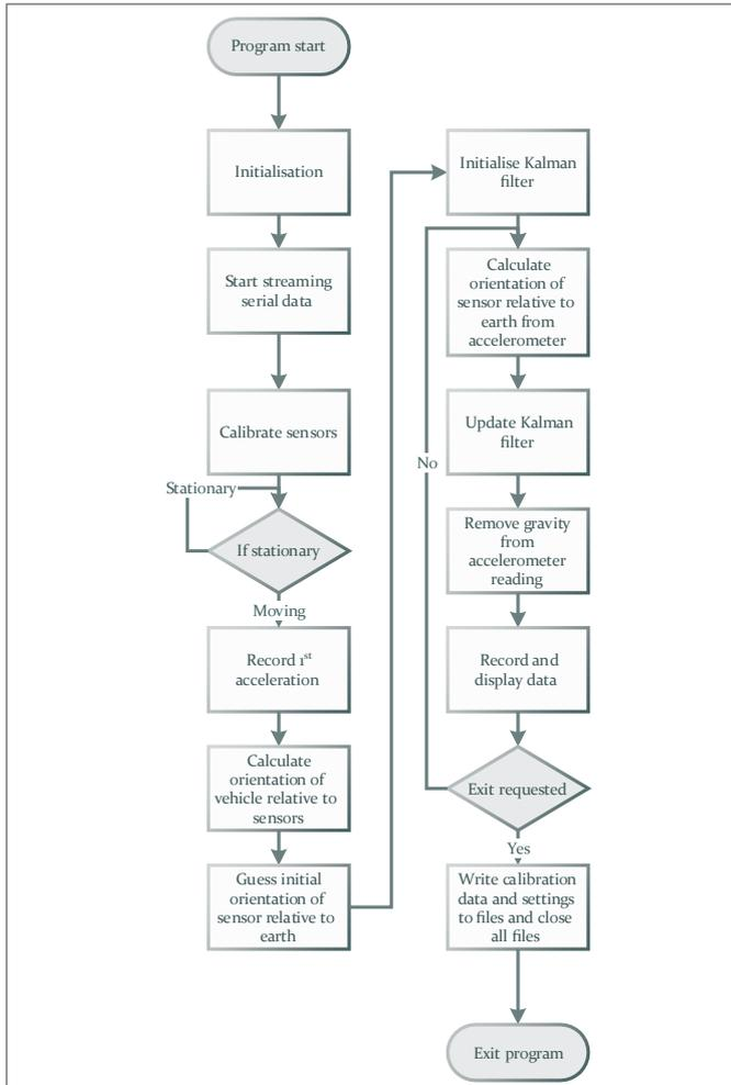
Figure 2: A flowchart illustrating the basic program operation
