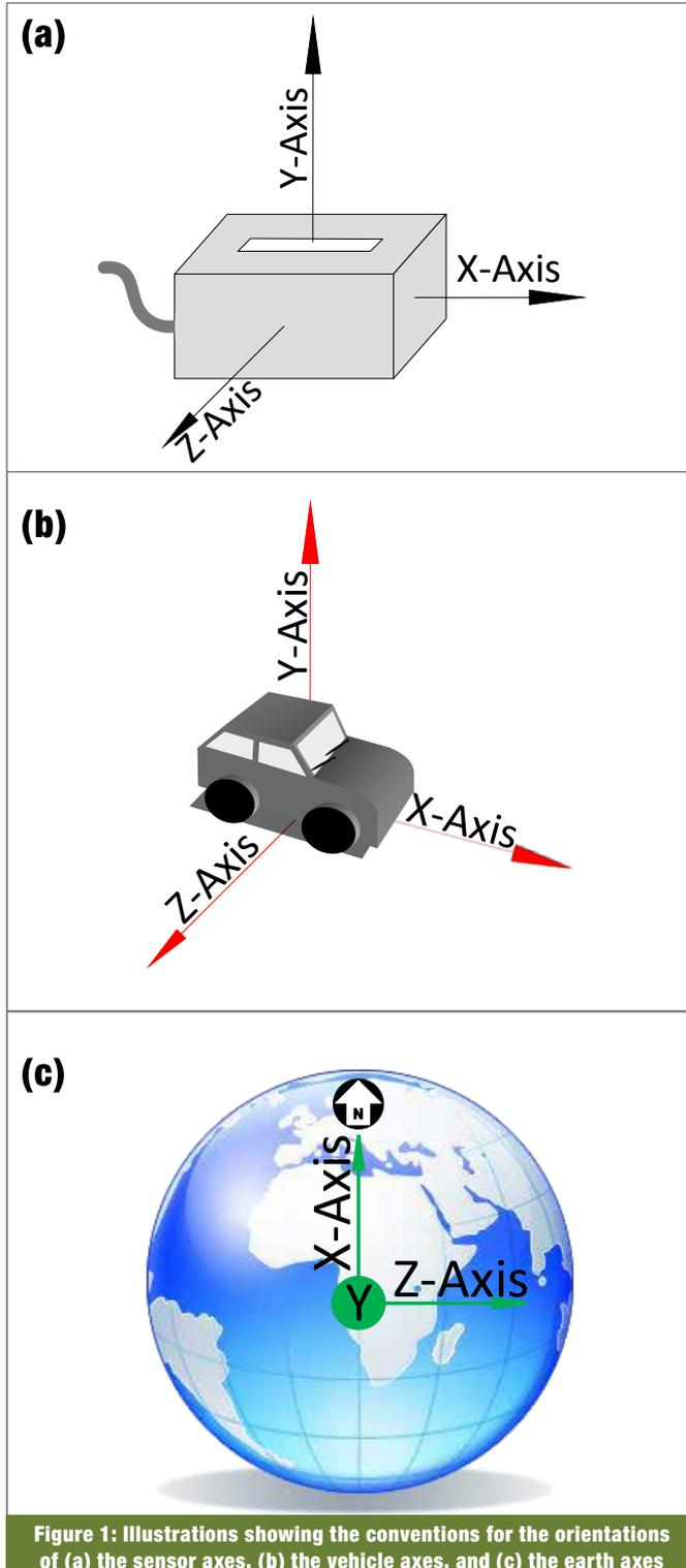
Figure 1: Illustrations showing the conventions for the orientations of (a) the sensor axes, (b) the vehicle axes, and (c) the earth axes
