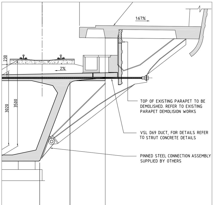
**Figure 4: Structural system for strut connections, transverse pre-stressing and slab supports**
