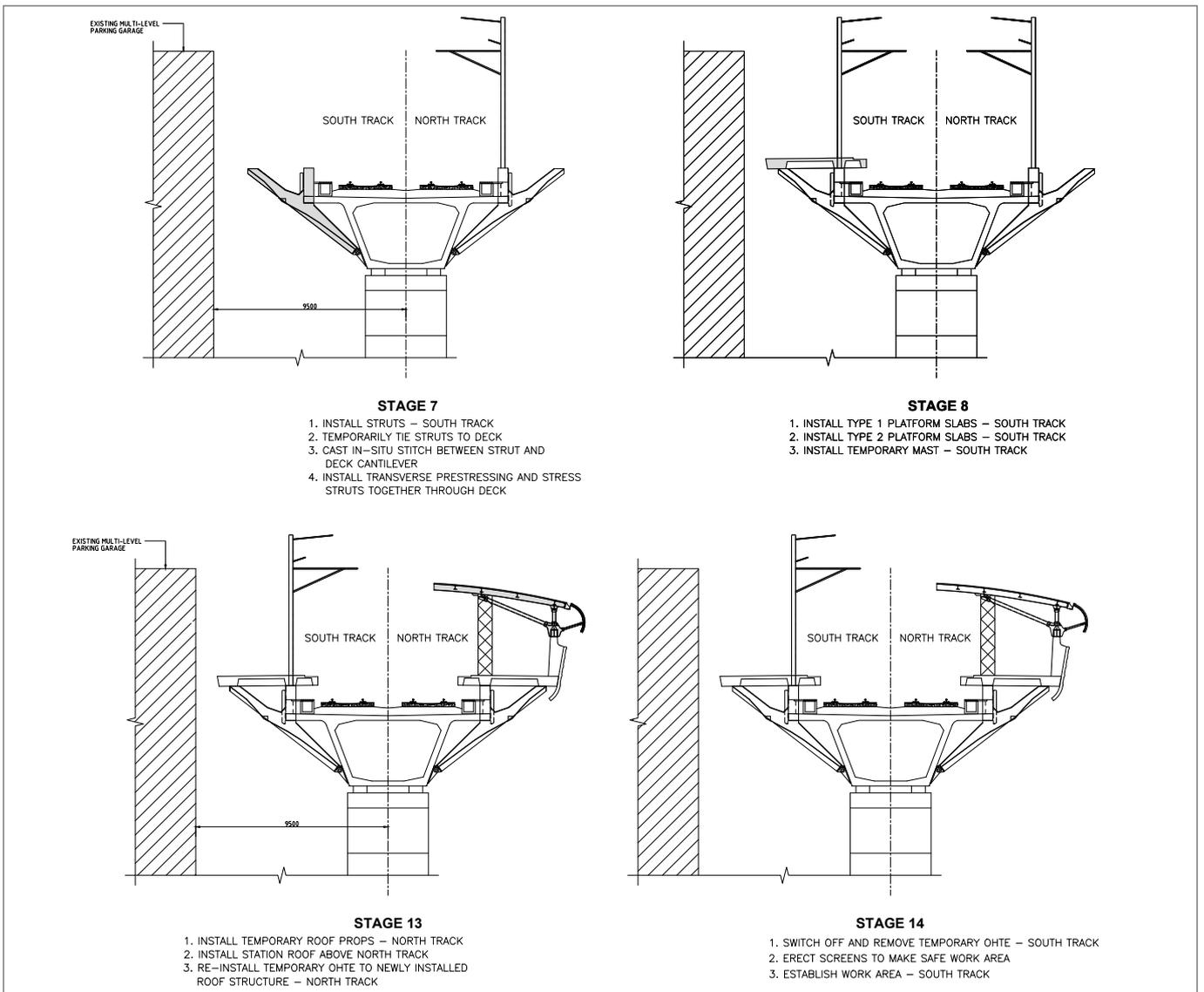
**Figures 8: Typical stages of construction, illustrating the temporary propping and temporary OHTE relocation arrangements**
