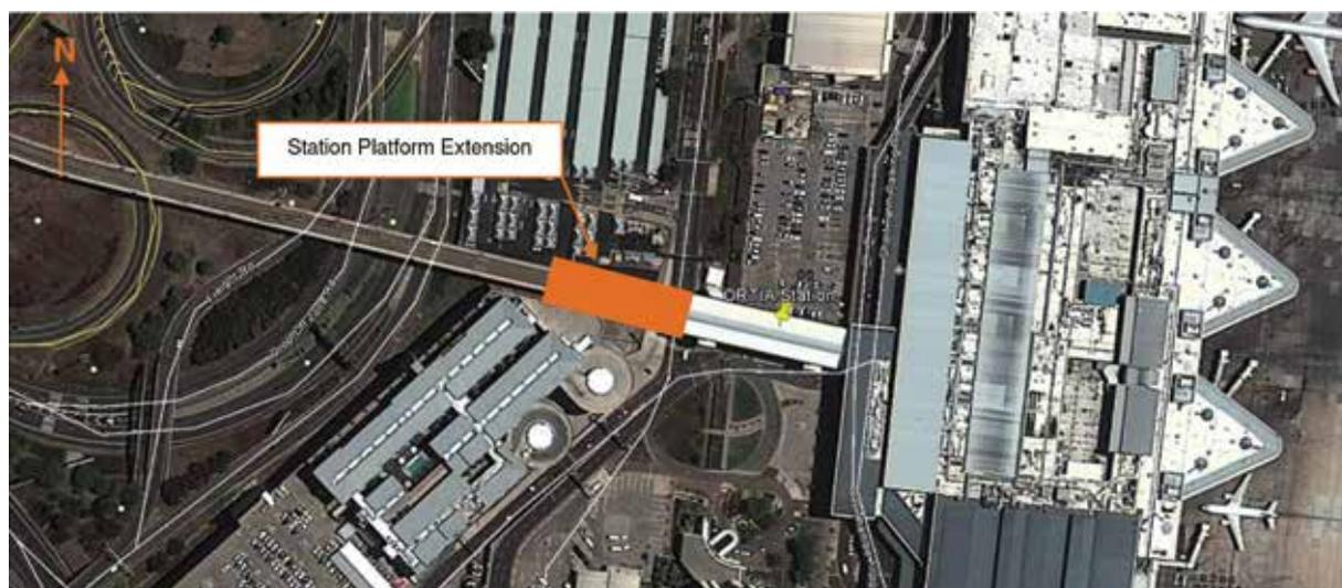
Figure 1: Satellite imagery of the extension to the OR Tambo International Airport Station
