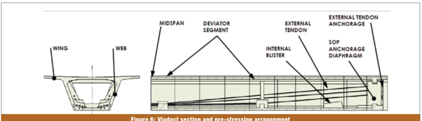
Figure 6: Viaduct section and pre-stressing arrangement
