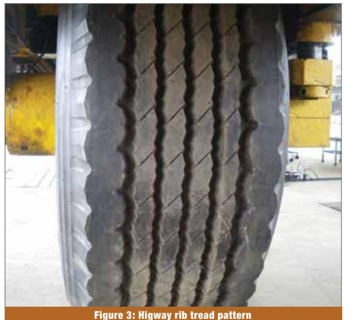
Figure 3: Highway rib tread pattern
