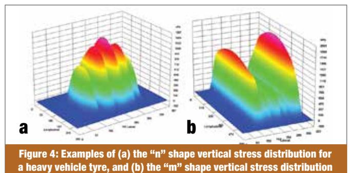
Figure 4: Examples of (a) the "n" shape vertical stress distribution for a heavy vehicle tyre, and (b) the "m" shape vertical stress distribution
