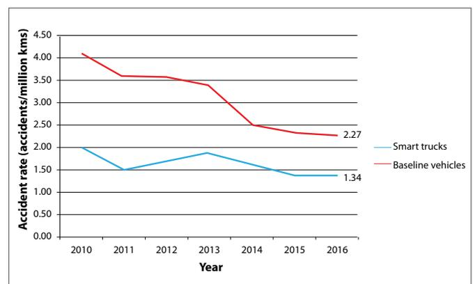
Figure 1: Accident rates for smart trucks and baseline vehicles
