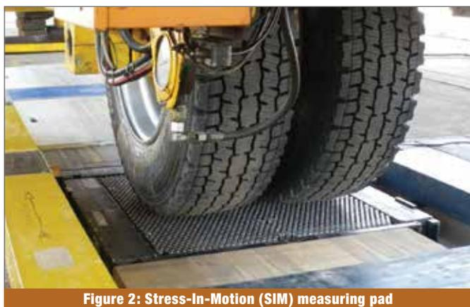
Figure 2: Stress-In-Motion (SIM) measuring pad
