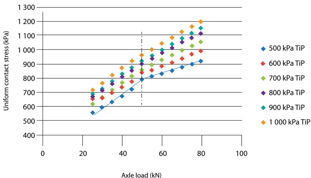
**Figure 5: Axle load versus uniform contact stress for Tyre 8 (315) at various tyre inflation pressures (TiP)**
